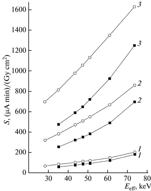
Fig. 2. Sensitivity of the  $\text{Cd}_{0.9}\text{Zn}_{0.1}\text{Te}$  detector as a function of the X-ray effective energy for a bias voltage of (1) 100, (2) 250, and (3) 400 V.
