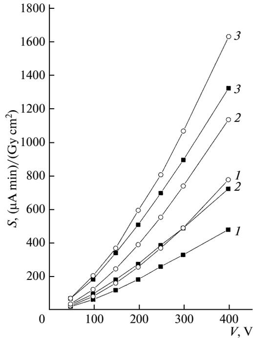
Fig. 3. Sensitivity of the  $\text{Cd}_{0.9}\text{Zn}_{0.1}\text{Te}$  detector as a function of the bias voltage for an effective X-ray energy of (1) 35, (2) 61, and (3) 72 keV.
