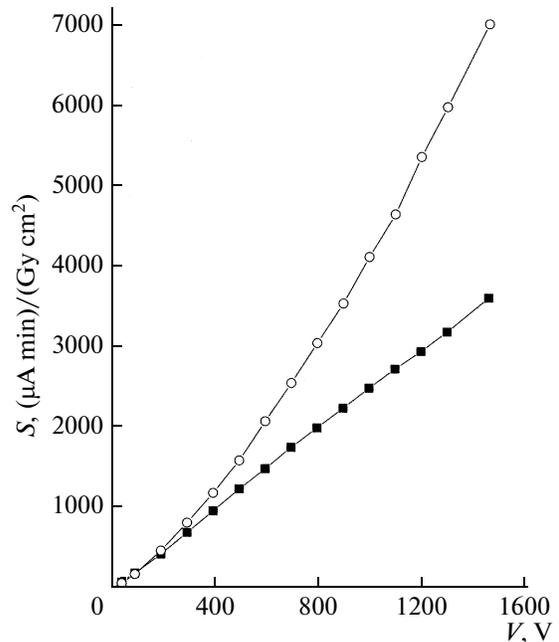
Fig. 4. Sensitivity of the detector as a function of the bias voltage for an effective X-ray energy of 61 keV.
