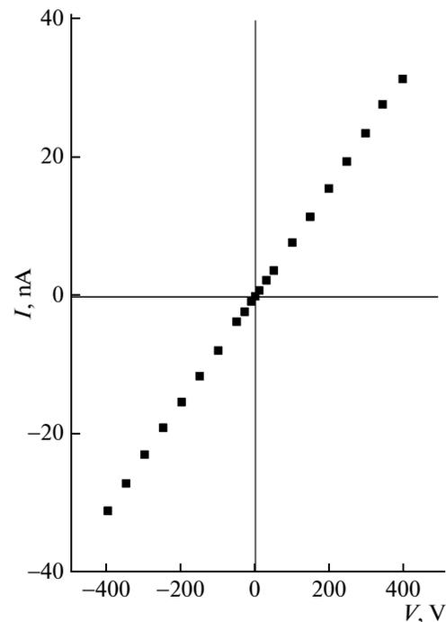
Fig. 1. Typical  $I$ – $V$  characteristic of the  $\text{Cd}_{0.9}\text{Zn}_{0.1}\text{Te}$  detector.
